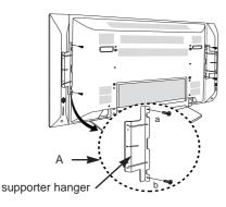
Assemble the monitor to speaker with using the supporter hanger and bolt. As shown above A, Assemble the a, b to the TV with using the bolt.
